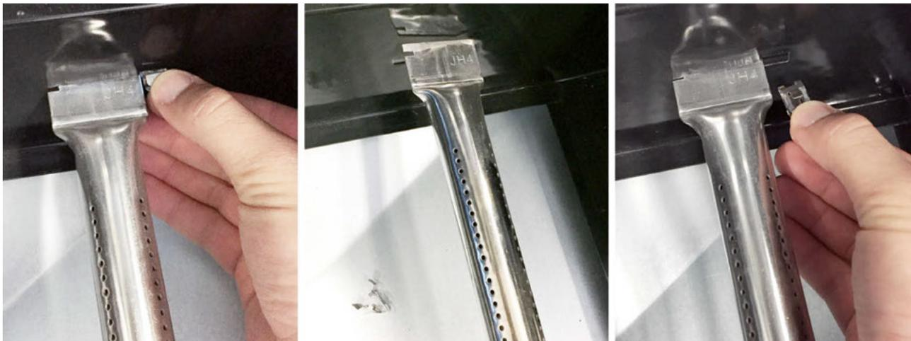
2. repeat step 1, from right side to left side to remove main burner and transmission frame, until remove the broken one.
